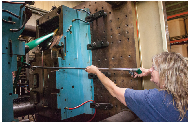
Left: Robotic technology helps streamline production and reduce costs. Right: Grabbing tools are an easy solution for removing tools that are hard to reach.
